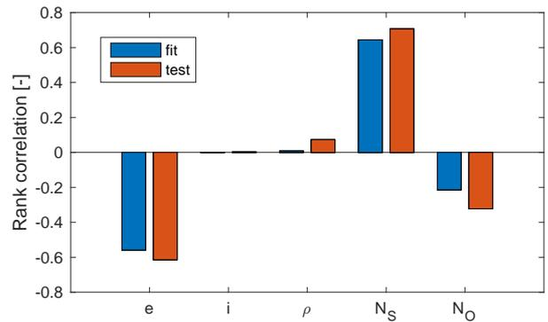
Figure 4. Sensitivity of orbit fit and propagation to the eccentricity  $e$ , inclination  $i$ , density  $\rho$ , number of stations  $N_s$ , and number of observations  $N_o$ .
