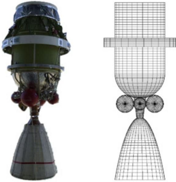
Figure 2. True and modelled Delta-K rocket body [11].
